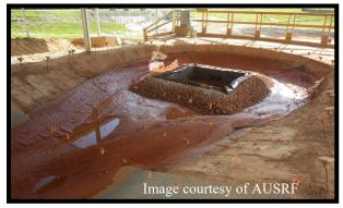
A drop inlet protection demonstration at the AUSRF
