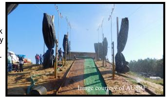
A rainfall simulator at the AUSRF with erosion control blanket demonstration
