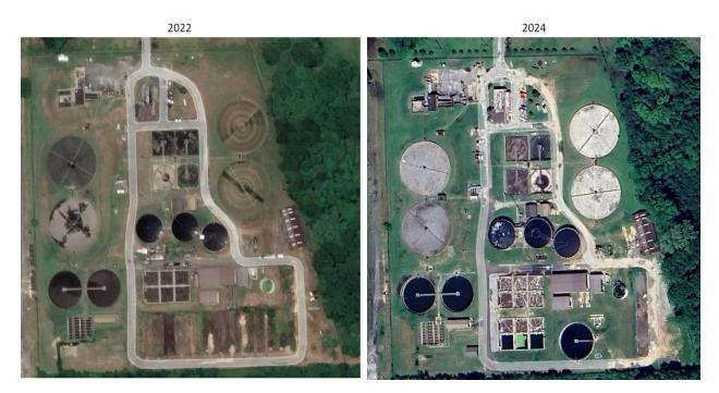
3. Currently, construction continues and the facility's four primary clarifiers are undergoing a complete and total overhaul. The timeline of the project's completion is totally dependent upon the components' manufacturer and any challenges it may face regarding supply chain issues. The components have been ordered and the funds have been allocated for payment upon delivery.
